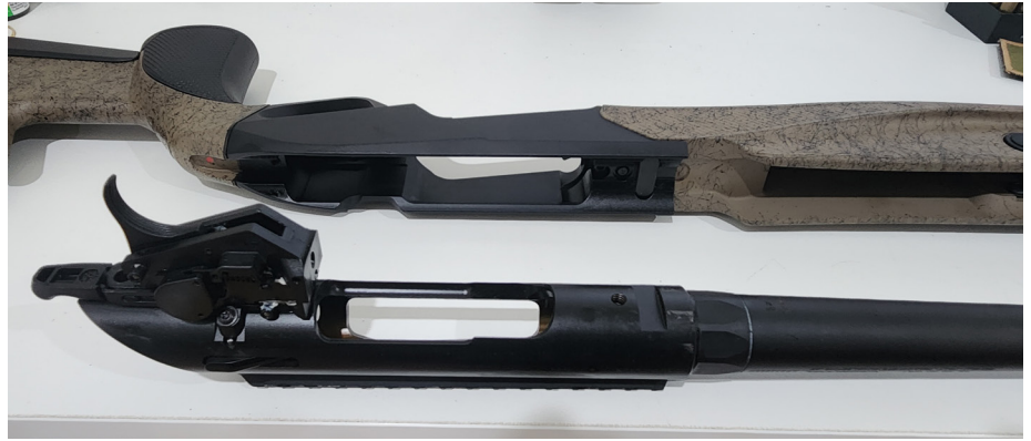
Cylindrical receiver mates precisely to the chassis by the large recoil lug and machined recess. Note large hexagonal barrel nut.
