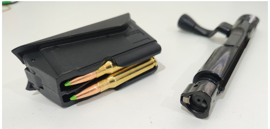
Dual-stack magazine and Lupo's tri-lug bolt with large claw extractor.
