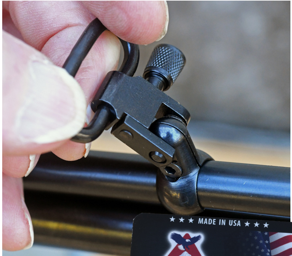
Fit the QD swivel to the tube magazine stud and job done.
