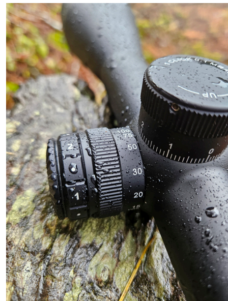
Above: Battery, illumination and parallax adjustment. Left: The scope passed the 'box' test with flying colours.
