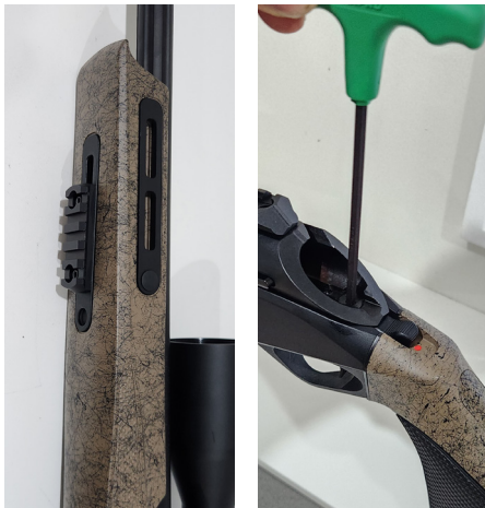
Left: Several M-Lok fittings allow for many accessory attachments; Right: Interestingly, rear action screw tightens from the top.
