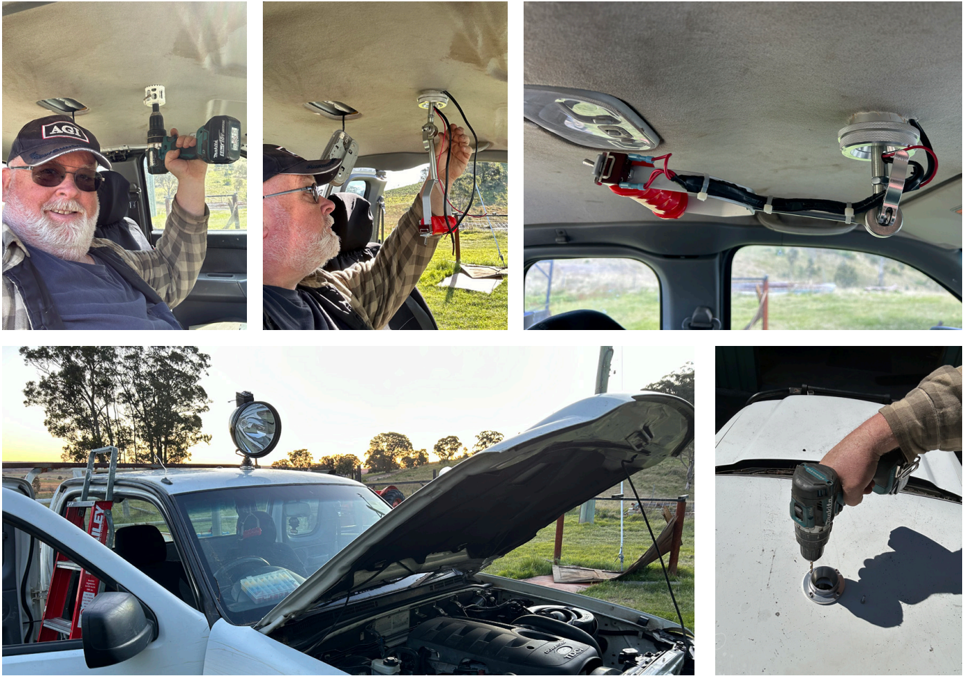
Clockwise from top: Daniel ready to drill through lining and roof; Daniel turns his hand to auto electrician, wiring up the spotlight remote handle; The Quick-Draw remote handle folds away neatly when not in use; Drilling the retention holes and dropping the bolts in as you go keeps everything aligned; Daniel chose to connect the spotlight direct to the battery via an Anderson plug.
