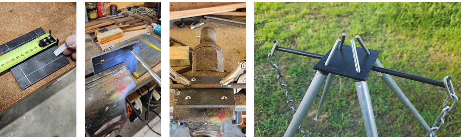
Clockwise from left: Marking holes on steel head plate; Drilling holes on the head plate; Preparing to weld chain bar to head plate; Completed and assembled head plate, poles and gong chain; Pink porta-gong easily visible at 600m.
