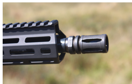
As tested the MPR Mini was fitted with an A1-style 'birdcage' flash hider, muzzle thread 1/2 x 28 should you wish to install other such devices.
