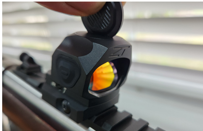
Battery is removed using the supplied tool.
