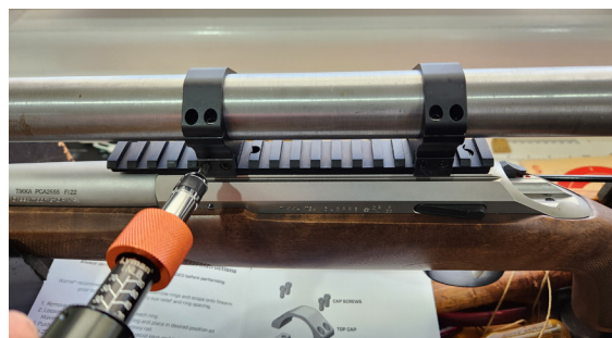
Below: Maxima rings on the 6.5 tightened to the correct torque using supplied instructions; The Vapor's large diameter single screws and thread; Maxima rings have remained accurate with many scopes at varying ranges (photo taken by remote means using tripod and timer).
