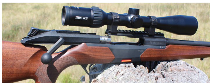
From top: The removable trigger pack features three-position adjustment from roughly 2-4lbs; The multi-lugged bolt head changing the orientation by 180 degrees switches the side to which the rifle ejects (cases always eject away from the plunger towards the extractor); With the exception of the scope rail interface the action is totally open. You can see through one side to the other.
