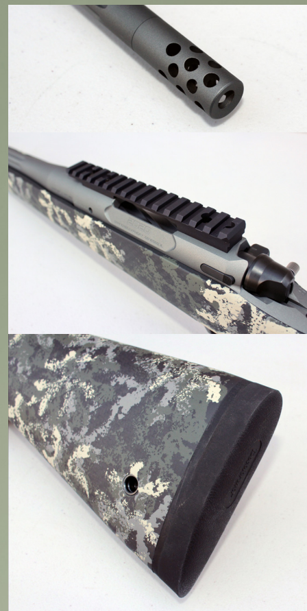
Radial muzzle brake comes fitted as standard but can be removed; Alloy Picatinny rail fitted as standard makes scope-fitting a breeze; Pachmayr Decelerator pad is another nice feature.
