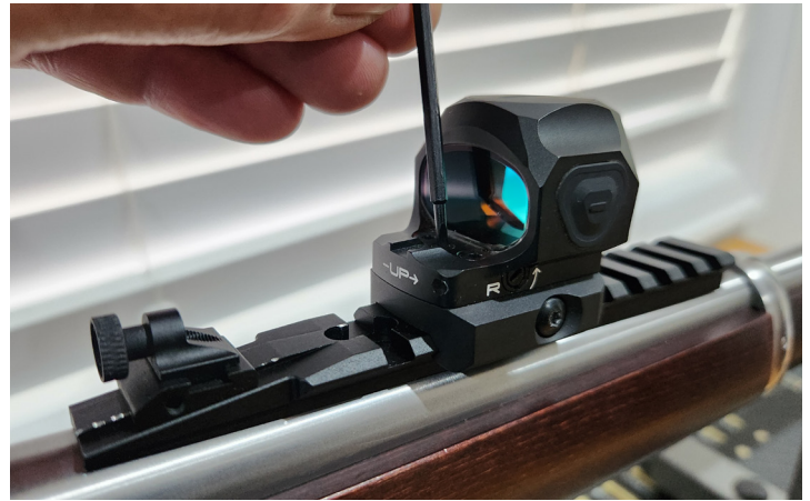
Elevation and windage adjusted easily using the supplied tool.
