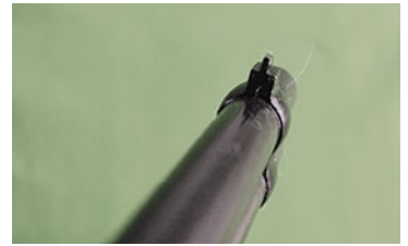
THE FRONT SIGHT IS A PISTOL-STYLE PARTRIDGE SQUARE BLADE.
