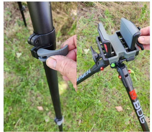
CAMMING TOGGLE LOCKS THE LEG POSITION; THE RUBBER PADS AND HEAVY DUTY CLAMP ARE WHAT MAKES THE DEATHGRIP (NOTE LARGE DIAMETER GUIDE PINS AND THREADED TIGHTENING SHAFT).
