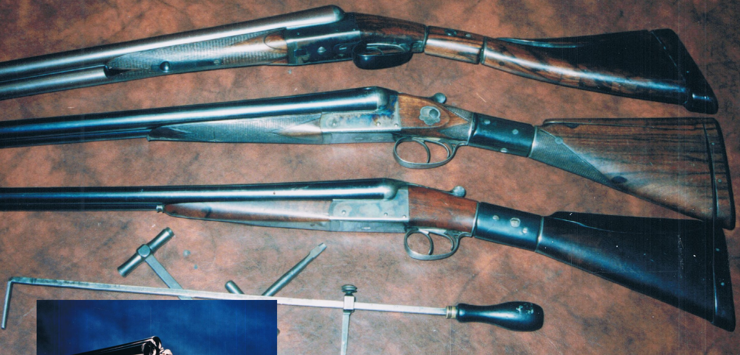
JOHN DICKSON & SON GUNS WITH LENGTH OF PULL GAUGE AND ADJUSTMENT TOOLS.
