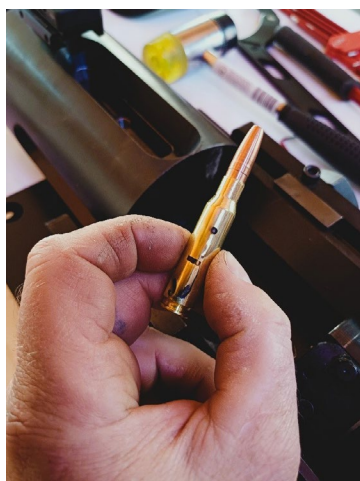
ARES' ROOSTER COUNTER-DRONE ROUND, DESIGNED TO DISINTEGRATE AFTER A CERTAIN DISTANCE TO MAXIMISE HIT PROBABILITY AND MINIMISE RISK TO CIVILIANS. THIS ISN'T SOMETHING SPORTING SHOOTERS WILL EVER GET TO TRY BUT IS INDICATIVE OF THE INNOVATION IN AUSTRALIA'S MUNITIONS SECTOR.
