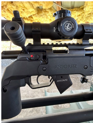
FROM TOP: ADJUSTMENT KNOBS FOR THE CHEEKPICE ARE RECESSED INTO THE STOCK. ALSO NOTE QD SLING CUP; THE EXPOSED COCKING INDICATOR GIVES BOTH A VISUAL AND TACTILE REFERENCE TO THE RIFLE'S STATUS; ALL FIRE CONTROLS ARE EASY TO ACCESS AND OPERATE.
