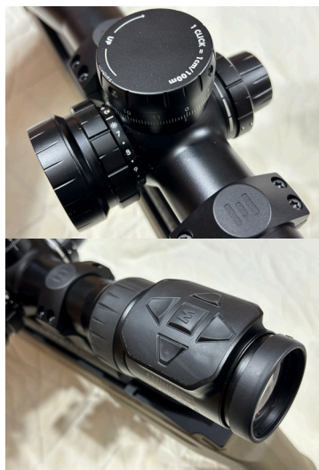
MAIN ELEVATION TURRET HAS CLICK ADJUSTMENTS AT A 1CM/100M VALUE AND, ON THE LEFT TURRET, THE ILLUMINATION HAS AN OFF POSITION BETWEEN EACH OF THE 11 BRIGHTNESS SETTINGS; MOUNTED ATOP THE OCULAR HOUSING IS A CONTROL PAD, THE ERANGER 8'S BALLISTIC COMPUTER.
