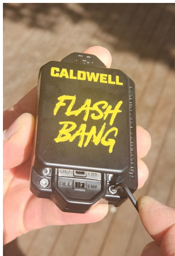
AN ALLEN TOOL IS USED TO REMOVE THE BACK COVER FOR BATTERY INSTALLATION. ON/OFF SWITCH SHOWN.
