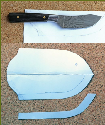
USE YOUR KNIFE AS A TEMPLATE TO DRAW A PATTERN FOR THE SHEATH AND WELT. THE INNER LINE ON THE SHEATH PATTERN INDICATES LOCATION OF THE WELT.
