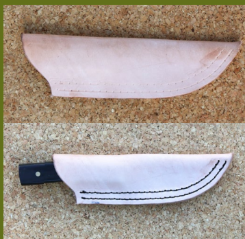
MARK STITCH LINES PRIOR TO SEWING. THE POINTS ON EACH STITCH LINE ARE EQUIDISTANT AND INDICATE WHERE A HOLE SHOULD BE TO ACCOMMODATE NEEDLES AND THREADS WHEN SEWING. (JOHN SEWS HIS SHEATH ON HIS HAND-OPERATED SEWING MACHINE, A MUCH QUICKER AND TIDIER PROCESS THAN HAND SEWING).
