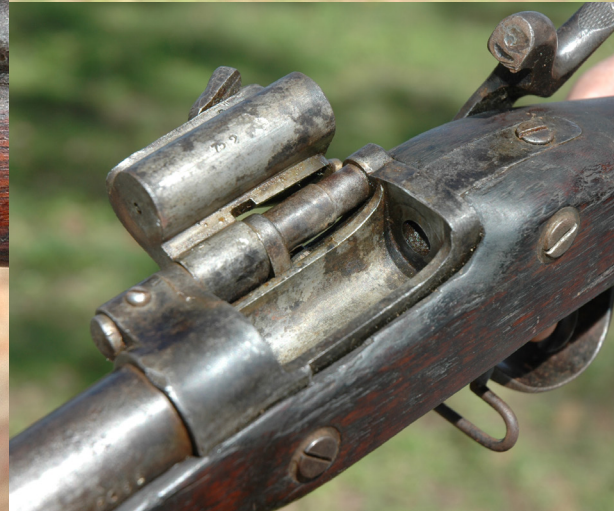
THE CONVERSION FROM A MUZZLELOADER TO BREECH LOADER WAS A BRILLIANT INVENTION, THIS MODEL MARKED 'SPRINGFIELD 1862.'; BREECH BLOCK SWINGS OUT TO ALLOW REMOVAL OF AN UNFIRED ROUND OR FIRED SHELLS; OPEN BREECH OF THE SNIDER CONVERSION ON THE ENFIELD MUSKET.
