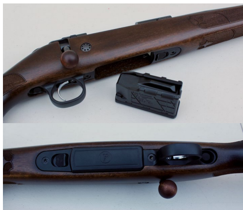
DETACHABLE BOX MAGAZINE HOLDS FIVE ROUNDS IN A DOUBLE-STACK MANNER; THE MAGAZINE RELEASE BUTTON IS LOCKABLE BY SLIDING IT FORWARD.
