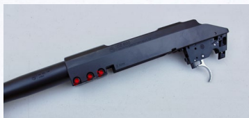
SPLIT FRONT RECEIVER WITH THREE BARREL-RETAINING NUTS.
