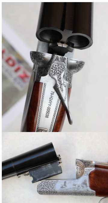
CLOSE-UP OF THE BARRELS DROPPED, EXPOSING THE SPLIT EJECTORS; THE BARREL LUMP WHICH ROTATES THE BARRELS AT THE FRONT AND LOCKS THEM TO THE RECEIVER VIA THE REARWARD BITE.
