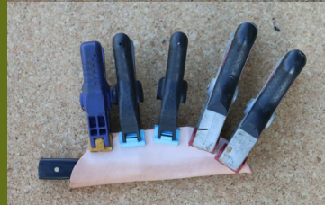
FOLD THE LEATHER READY FOR THE WELT TO BE GLUED IN PLACE. CLAMP TOGETHER WITH THE KNIFE INSIDE TO ENSURE IT FITS AS IT SHOULD.
