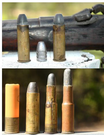
THE RIMMED .577 ENFIELD CARTRIDGE IS HUGE. THEY WERE INITIALLY ISSUED IN A COILED BRASS FOIL VERSION; THE .577 ENFIELD CAN BE RELOADED WITH 20-GAUGE SHOTSHELLS. THE .577 ROUND IS HUGE COMPARED TO THE COILED BRASS FOIL .450/.577 CASE AND LATER BRASS .450/.577 ROUND WHICH REPLACED IT.
