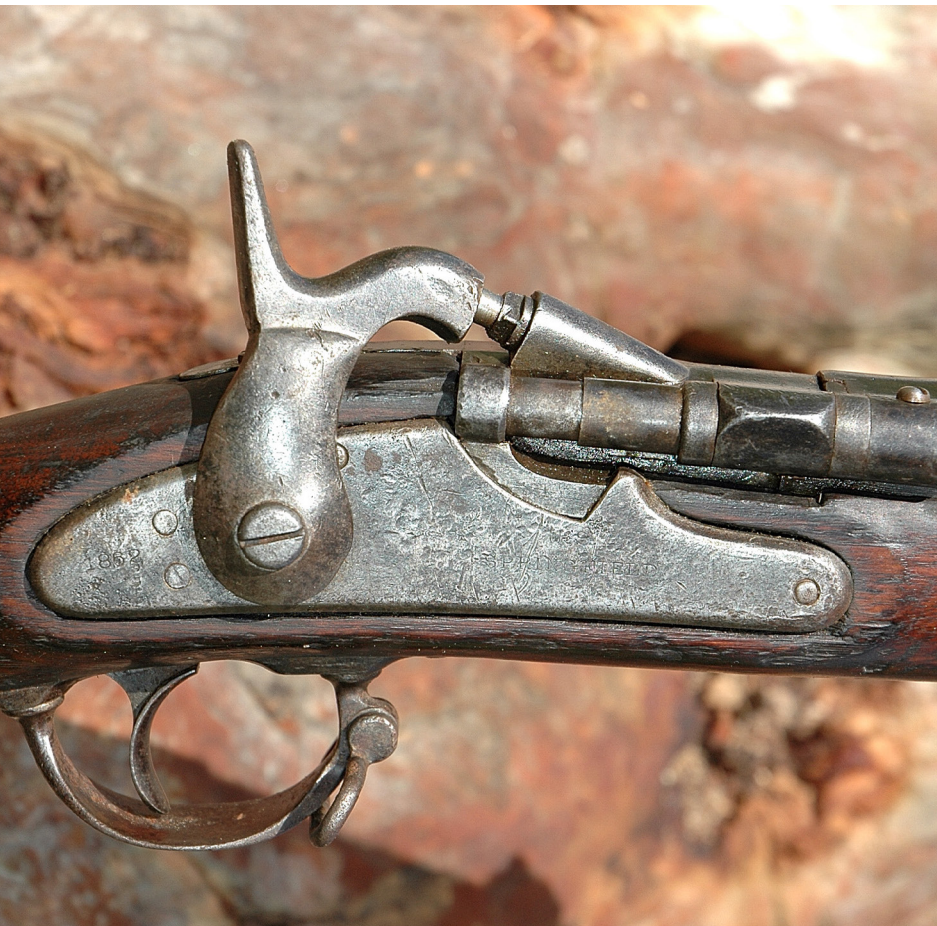
THE CONVERSION FROM A MUZZLELOADER TO BREECH LOADER WAS A BRILLIANT INVENTION, THIS MODEL MARKED 'SPRINGFIELD 1862.'; BREECH BLOCK SWINGS OUT TO ALLOW REMOVAL OF AN UNFIRED ROUND OR FIRED SHELLS; OPEN BREECH OF THE SNIDER CONVERSION ON THE ENFIELD MUSKET.
