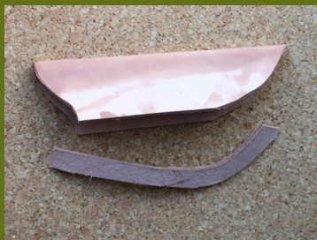
USE YOUR KNIFE AS A TEMPLATE TO DRAW A PATTERN FOR THE SHEATH AND WELT. THE INNER LINE ON THE SHEATH PATTERN INDICATES LOCATION OF THE WELT.
