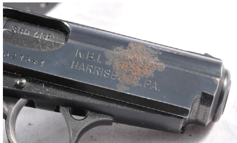
RUST AND CORROSION CAN BE A PROBLEM BUT LIGHT OILING HELPS PREVENT THIS.
