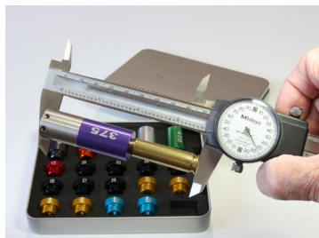
DIFFERENT TYPES OF BUSHING HOLDERS AND ANVIL BASES ARE AVAILABLE TO ATTACH TO YOUR CALIPERS. THIS VERSATILE TOOL LETS YOU MEASURE INDIVIDUAL BULLETS TO A POINT ON THE OGIVE.
