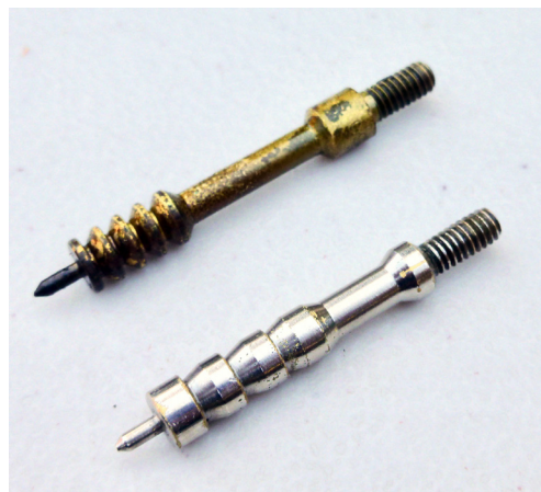
A BRASS .30-CALIBRE JAG (TOP) COMPARED TO A NICKEL-PLATED .30-CALIBRE JAG (BOTTOM). NOTE - THE NICKEL PLATING IS STARTING TO WEAR ON THE EDGES OF THE NICKEL JAG AND THE BRASS CORE CAN BE SEEN. TIME TO REPLACE WITH A NEW JAG.
