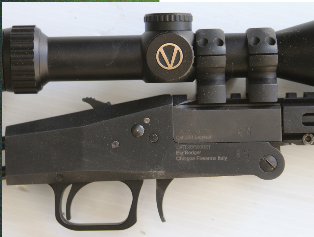
LEFT: BIG BADGER RECEIVER. THE LARGEST PIN IN THE CLUSTER OF ACTION PINS IS THE CROSS-BOLT SAFETY. NOTICE THE NARROW GAP BETWEEN HAMMER SPUR AND OVERHANGING SCOPE TUBE, NOT AN IDEAL SETUP.
