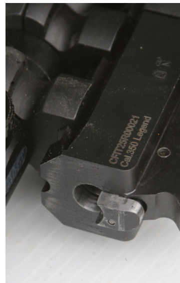
DEMI-BLOCK (BREECH END) SHOWING THE CHAMBER AND EXTRACTOR WITH THE ACTION LOCKING BLOCK ON THE BOTTOM.
