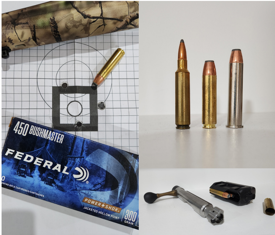
CLOCKWISE: APPROXIMATE 2MOA THREE-SHOT GROUPS AT 100M WERE CONSISTENT FOR THE 300-GRAIN FEDERAL POWER-SHOK LOADS; .450 BM CARTRIDGE FLANKED BY THE .284 WIN (LEFT) AND .45/70GOVT; THREE-LUG BOLT FOR SHORT BOLT THROW AND POLYMER THREE-SHOT DETACHABLE MAGAZINE.
