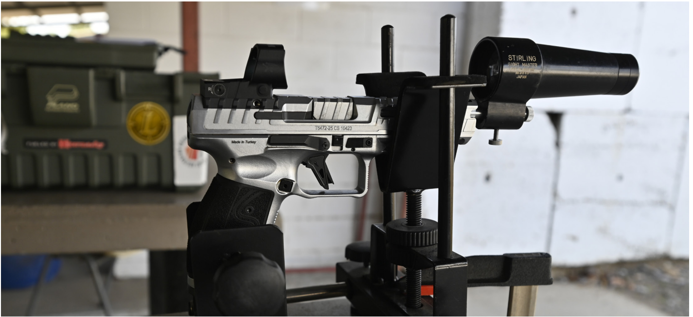
THE HYSKORE PISTOL REST MAKES SIGHTING-IN RED DOTS SIGHTS EASY, ESPECIALLY WHEN USED WITH A COLLIMATOR.
