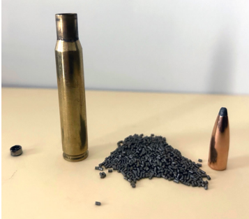
THE CONSUMABLES: PRIMER, BRASS CASE, POWDER AND PROJECTILE.
