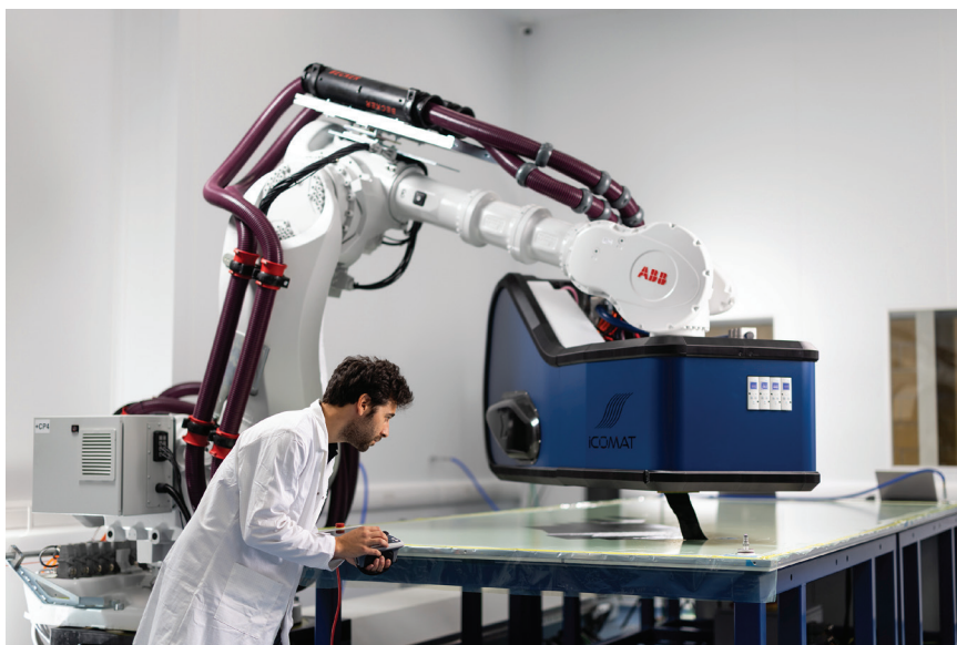
■ An engineer operates iCOMAT's rapid tow shearing (RTS) deposition head mounted on a six-axis ABB robot at the company's Gloucester facility. Source | iCOMAT
