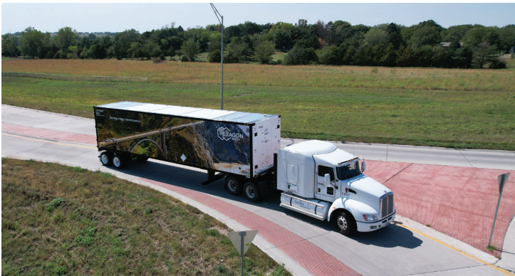
■ Hexagon’s Titan 510 Mobile Pipeline modules offer improved maneuverability and use thermoplastic composite (TPC) panels to cut nearly 2,000 pounds of weight for improved payload capacity. Source | Hexagon Composites
