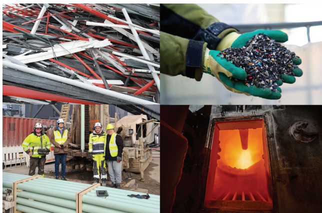
■ A partner in the KiMuRa project which collects, shreds and reuses composite waste in Finland in a cement co-processing plant (top left, clockwise), Exel Composites worked with customer Qheat to make sure its glass fiber composite pipes for geothermal heating (bottom left) can be reused in this way at their end of life (EOL). Source | CLIC Innovation, QHeat, Exel Composites
