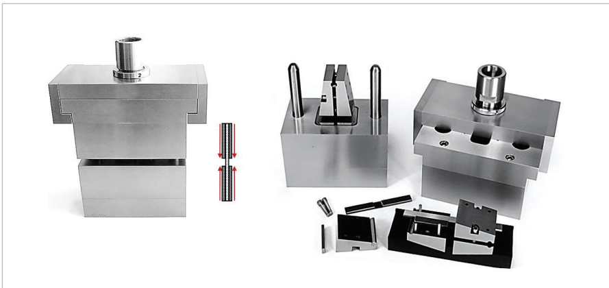
FIG. 1 ASTM D3410 IITRI compression test fixture and specimen loading. Source (All Images) | Dan Adams
