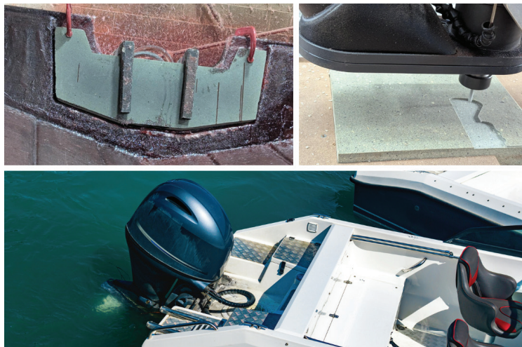
■ What started as an effort to reuse some of its own urethane foam scrap turned into a new side of RiversEdge Composites' business, manufacturing and selling transoms (top left image) and other board products made from recycled composite waste. Source | RiversEdge Composites (REC) (top images), Getty Images (bottom)
