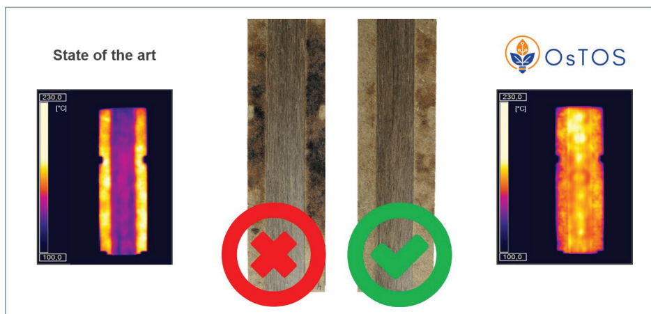
■ A comparison of conventional and OsTOS heating results demonstrate the latter's ability to intelligently preserve thermal consistency.
