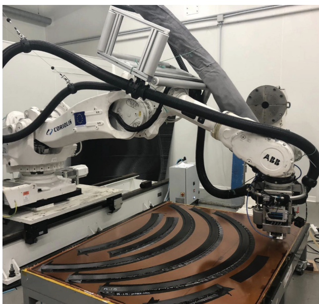
■ Avel's first TPC hydrofoil batten produced using the AFP process (top) and TPC qualification test articles being laid up for consolidation and characterization (bottom). Source | Oceania Bordeaux via Avel Robotics
