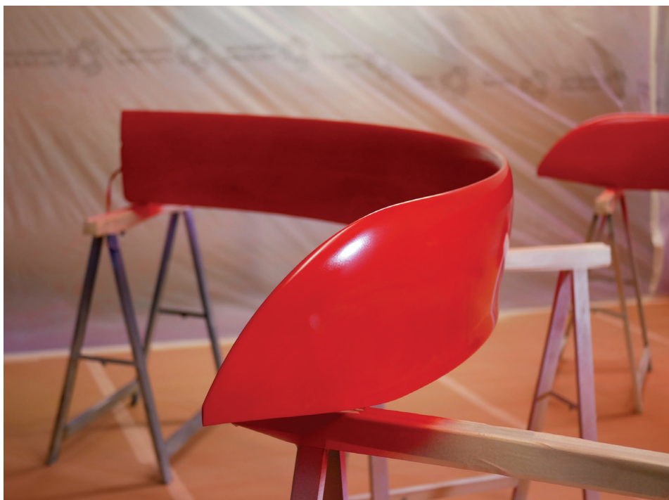
■ Freshly painted thermoplastic composite (TPC) hydrofoil for 754 manufactured by MiniLab. Source | Avel Robotics
