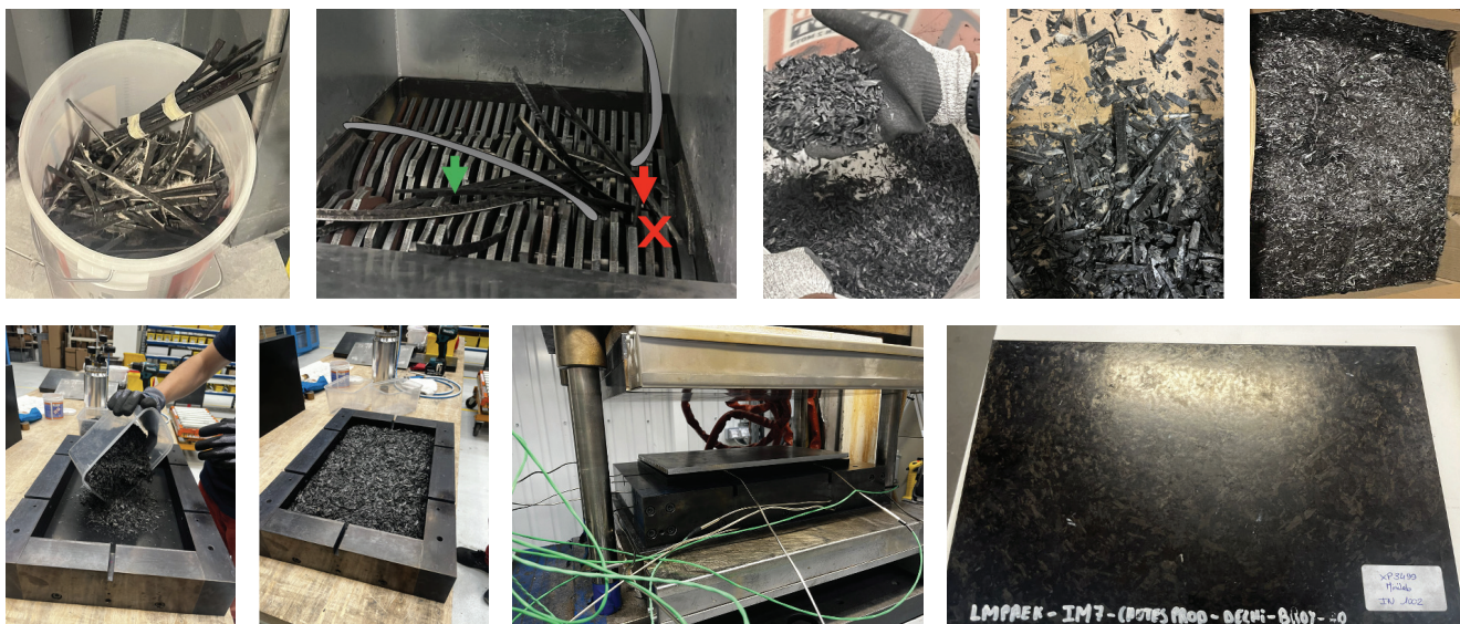
■ Recycled scrap converted to material for leading and trailing edges of a TPC hydrofoil. Source | Avel Robotics
