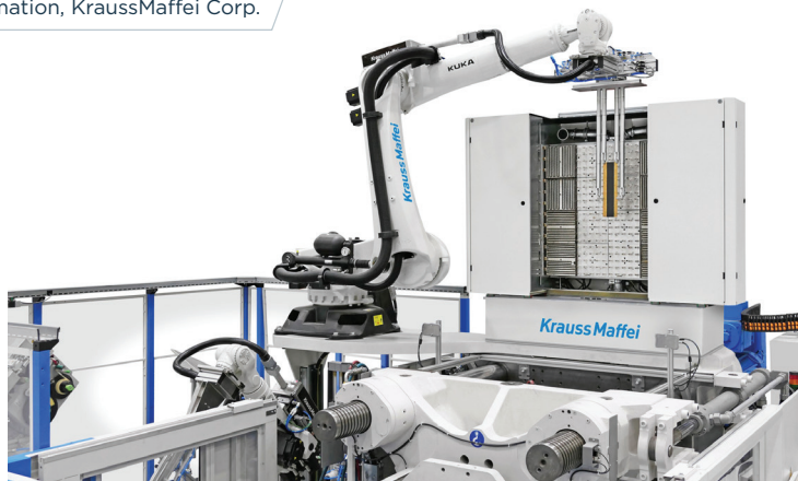
■ An IR oven with mixed IR-transmitters is installed here on a KraussMaffei injection molding machine. Source (All Images) | KraussMaffei
