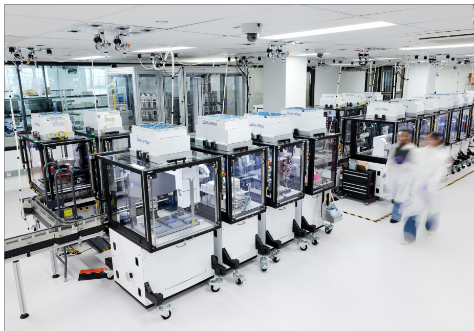
Automated lab foundry at Ginkgo Bioworks' Boston headquarters. Proprietary reconfigurable automation carts with a modular configuration are used to run diverse lab data generation workflows for different clients. [Ginkgo Bioworks]
