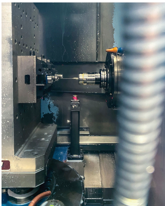
A Renishaw touch probe is used for in-process measurement of critical machined features for high-precision jobs.
