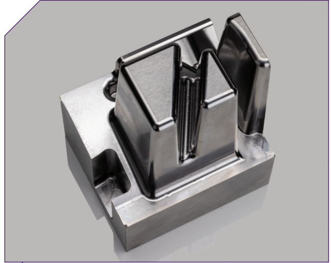
Long-reach tooling in demanding deep rib geometry, delivering smooth, consistent surface finish without polishing, demonstrating the impact of controlled tool paths and stable machining. Source (all images) CGS North America
