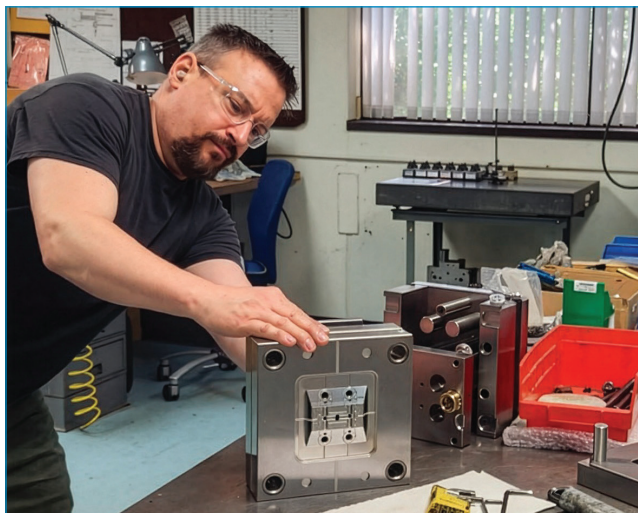
Installing ejector pins in a four-cavity mold, before setting up in the EDM to burn everything in place.
