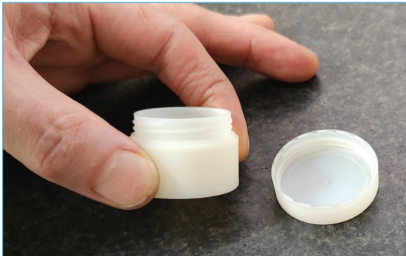
Jar and Lid made of PHA via a three-plate mold runner design. The mold uses cams for external threads and a helical spindle from Hasco for the internal threads of the lid.
