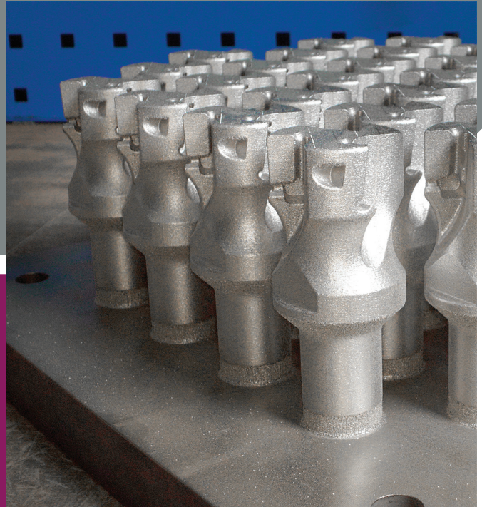
Batch production of end mills produced via 3D metal additive manufacturing. Source (all images): Iscar Metals
