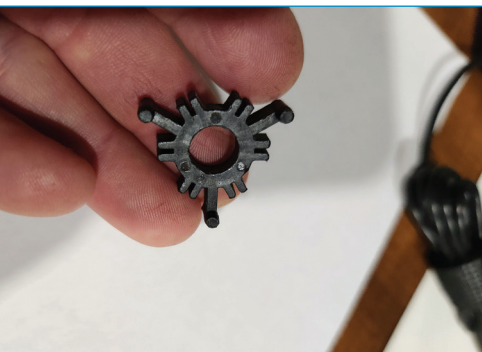
A four-cavity, star-shaped part packed into a small MUD frame. Source: Bob Novak
