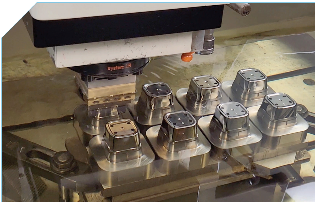
Burning ribs for an eight-cavity square dosage cup mold. Source (all images): Evolve Tool and Mold Design.
