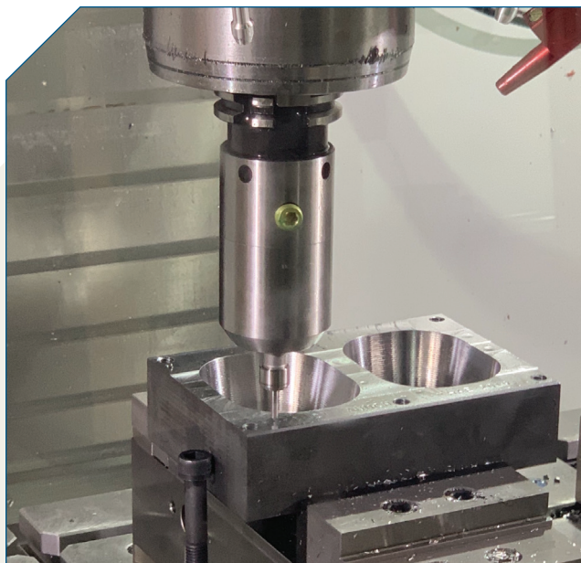
Add-on air-turbine spindles can be integrated with a range of CNC machines, including this five-axis machine. Here the spindle is milling at 65,000 rpm. Source (all images): Air Turbine Tools
