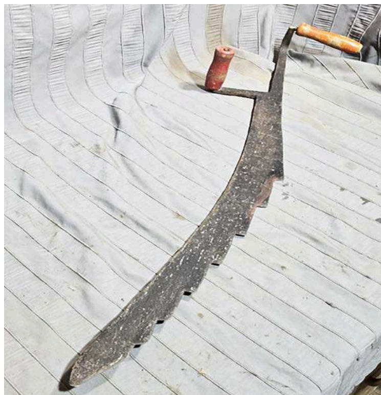
Some hay knives look like oversized bread knives with a long-serrated edge and handles offset from the blade.
