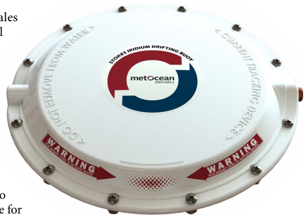
A MetOcean Stokes drifter. The compact drifting buoy is equipped with GNSS positioning, a sea surface temperature sensor, and Iridium satellite telemetry, enabling the buoy to transmit sensor and geo-positional location data in real time. Photo: MetOcean.
