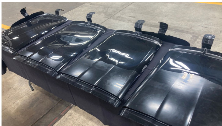
Demonstration parts molded at Omega. These parts have been intentionally short-shot with the in mold coating to illustrate the coating process, with progressively longer shots from right to left.
