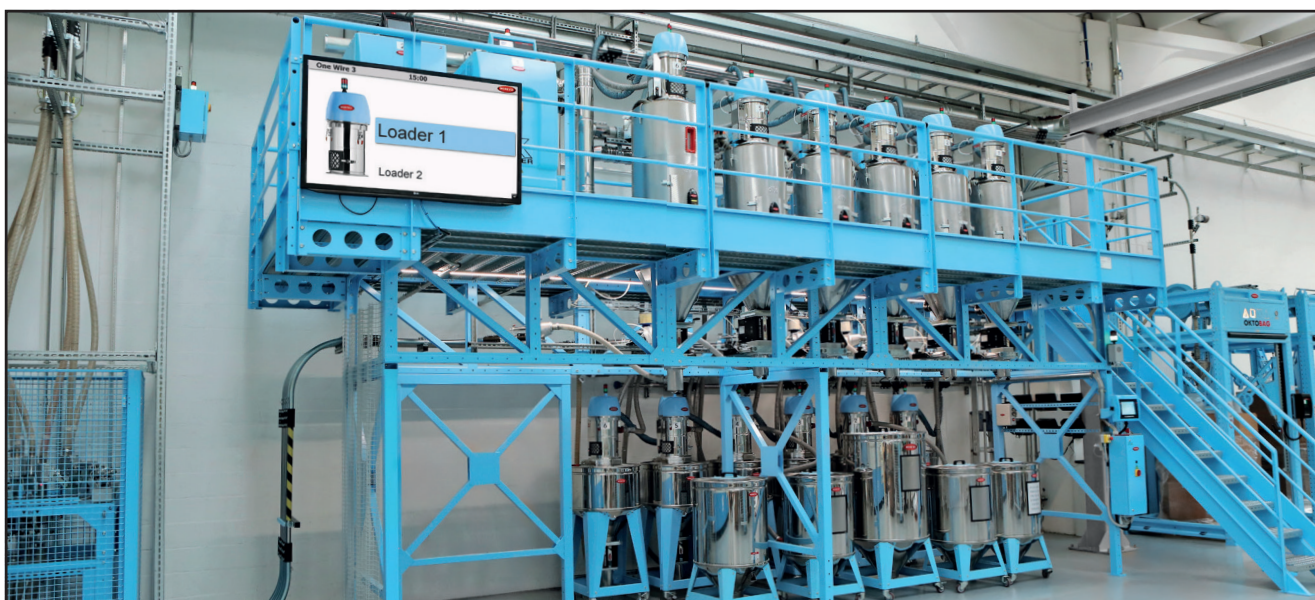
Completely Automated Material Handling and Central Drying Systems with Inline Moisture Analysis.
