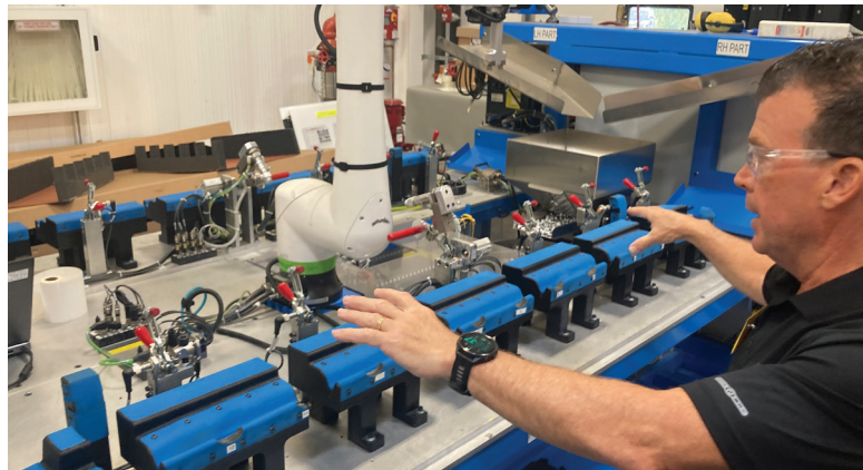
Greg DeFrancisco explains how the cobot station with custom fixturing is used to assemble finished parts.
