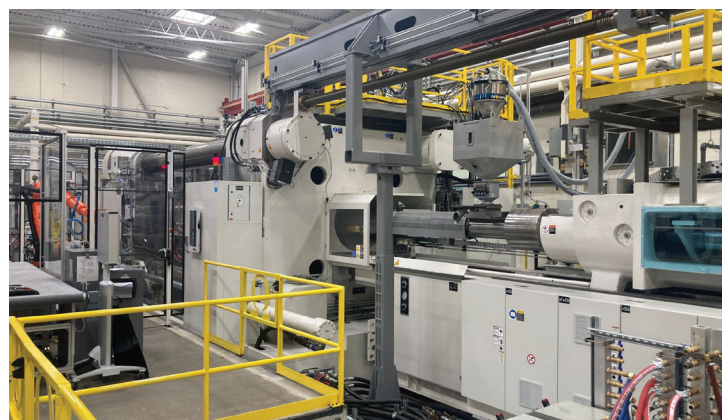
The 4500-kN (505 tons) KraussMaffei press outfitted for the Colorform PUR coating process.
