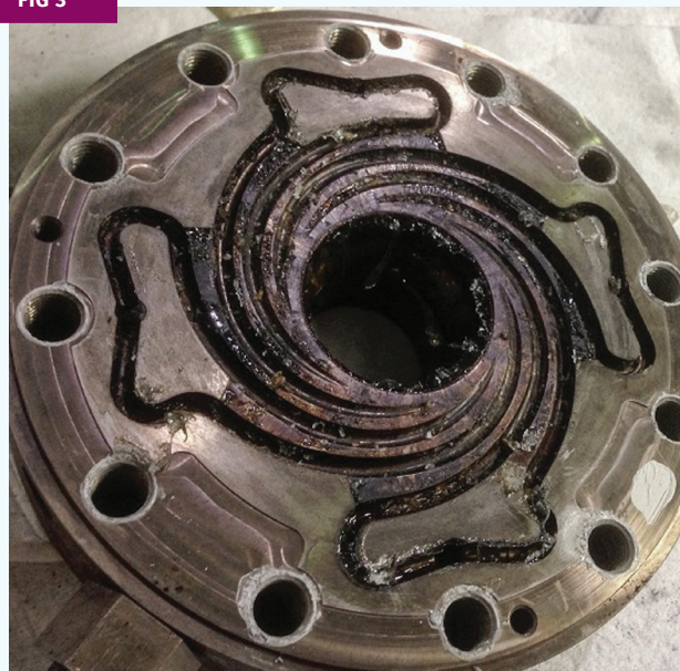
Stacked pancake die spiral flow channel (die split for cleaning).
