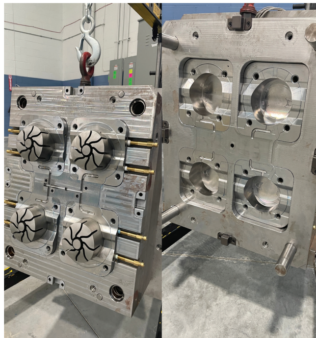
As part of an experiment, Atomic created this tool with various cooling technologies — human and AI designed, as well as regular and conformal — to test the efficiency of various methods.
