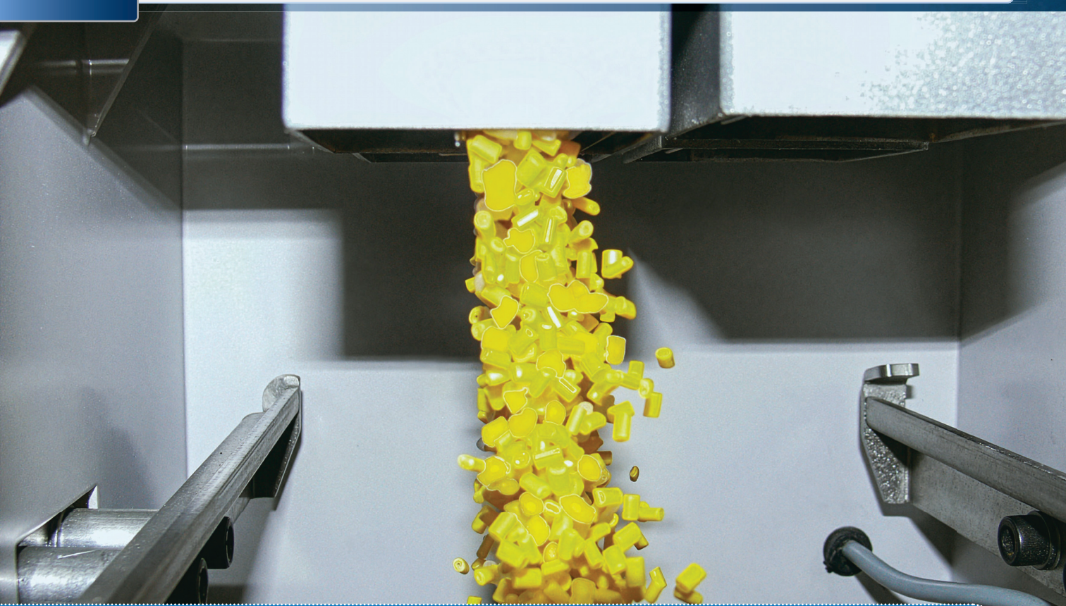
FIG 1: Color and additives can be free-flowing or non-free flowing (pulsing). Image shows the former. Source: Wittmann
