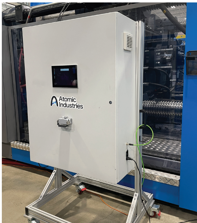
Atomic builds these press-side data-collection units to help it gather process information to feed back into its Nucleus software.
