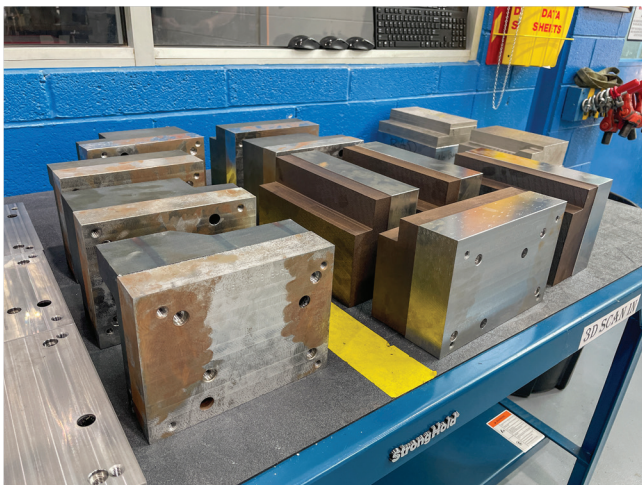
Atomic uses AI to help it design conformally cooled cavity inserts which are then 3D printed with Velo3D laser powder-bed fusion technology.
