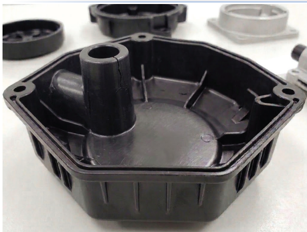
FIG 6A The cracked boss feature encountered when using the replacement material.
