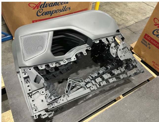
These automotive door panels were molded utilizing iMFLUX constant pressure technology, enabling use of six valve gates vs. eight.
