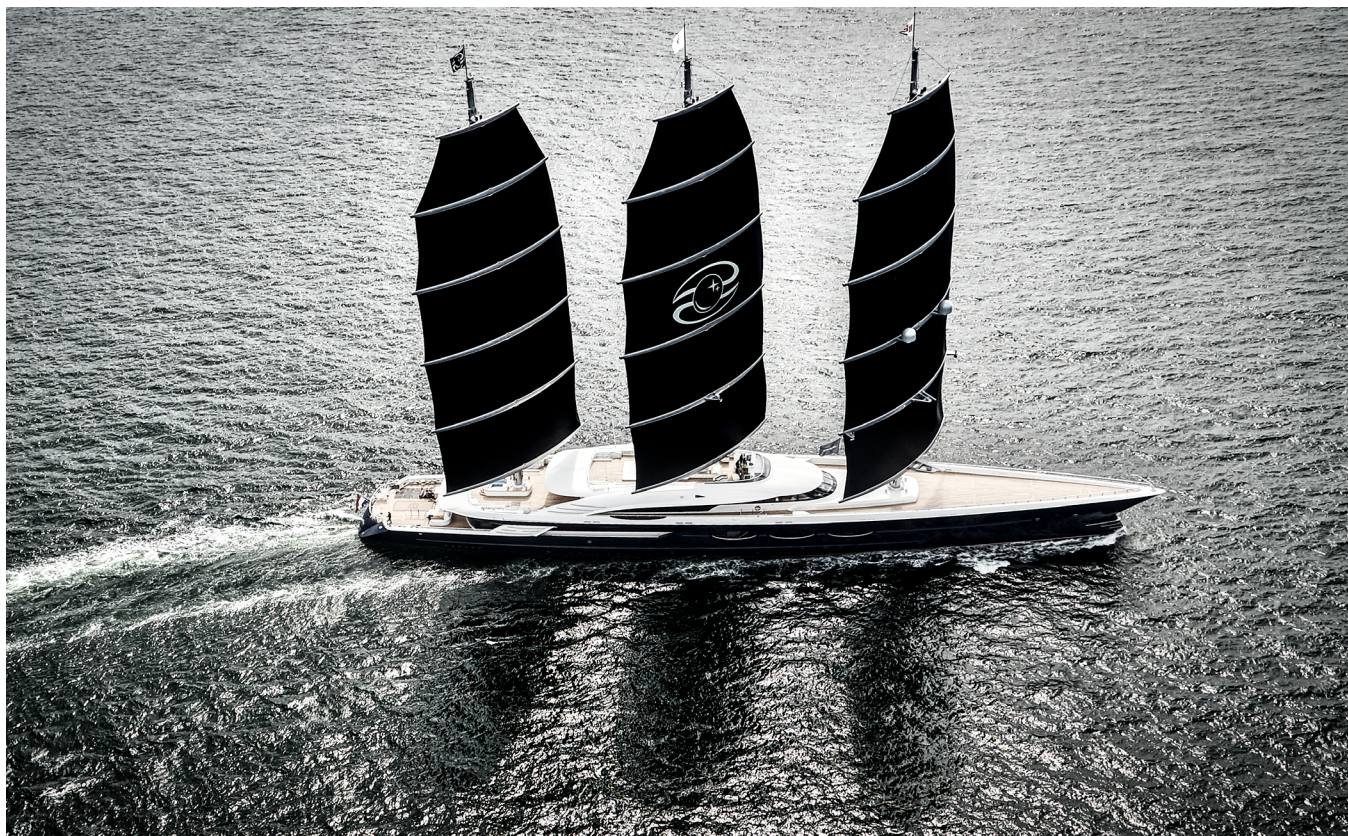
The 107m (351') Black Pearl, built by Oceanco in 2016, is driven by a Dykstra-designed DynaRig 25% larger than Maltese Falcon 's.
