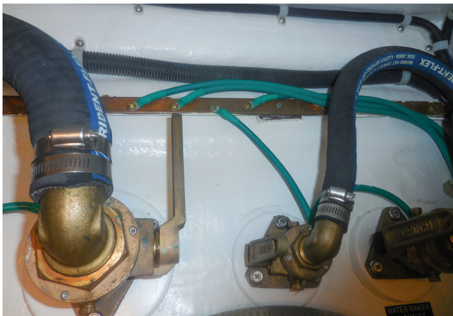
A bonding system connected to all underwater metal hardware and machinery protects them from stray-current corrosion by returning any fault current from onboard systems directly back to the battery.
