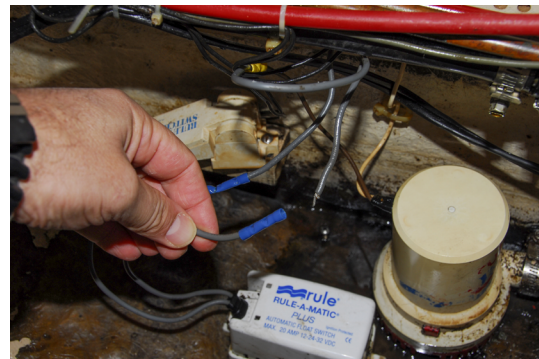
A common source of corrosive stray current in the bilge is pump wiring connections that are too close to the water and unprotected by waterproof heat-shrink tubing.
