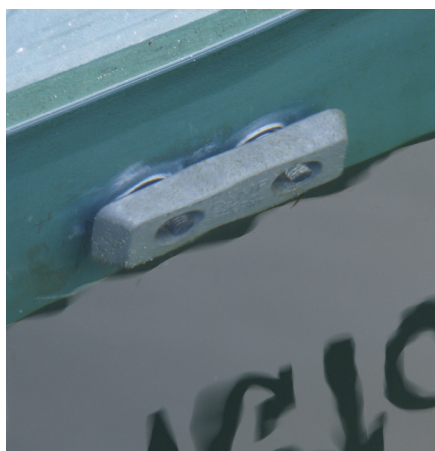
On a planing hull, the anode for an onboard bonding system mounts to the transom below the waterline.
