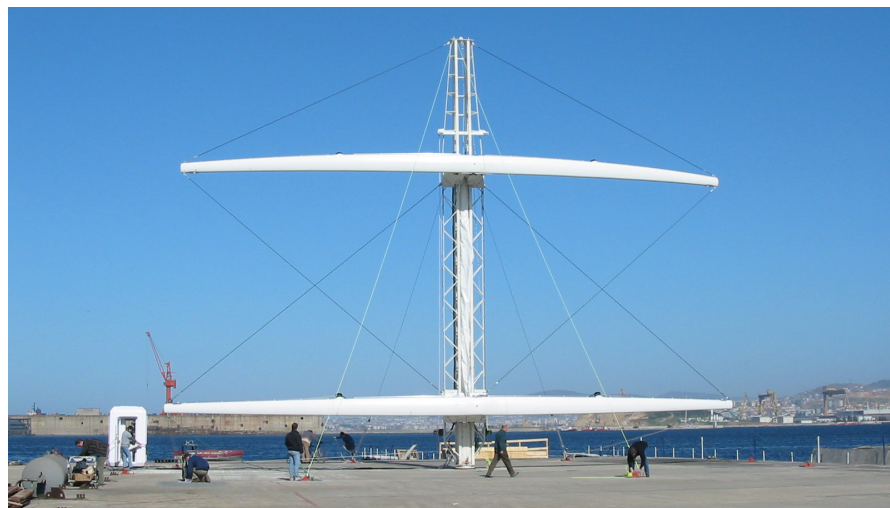
Full-size test of DynaRig mast, yards, sail, and control mechanism for Maltese Falcon in Turkey.
