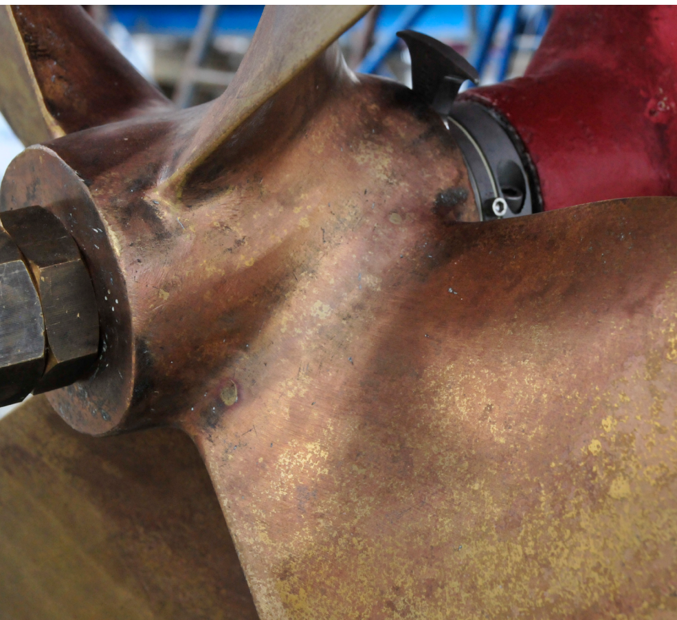
The telltale pink hue of dezincification in this propeller suggests a need for replacement or addition of sacrificial shaft anodes (zincs).
