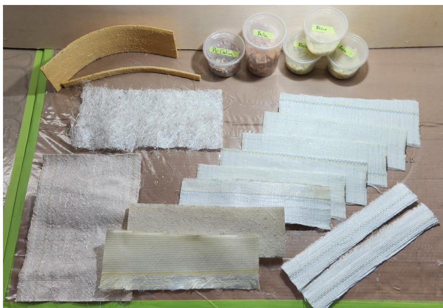
Above —All the components recovered from another blade section, this one built with nonrecyclable thermoset epoxy resin, using Resolve’s ReceTT process.
