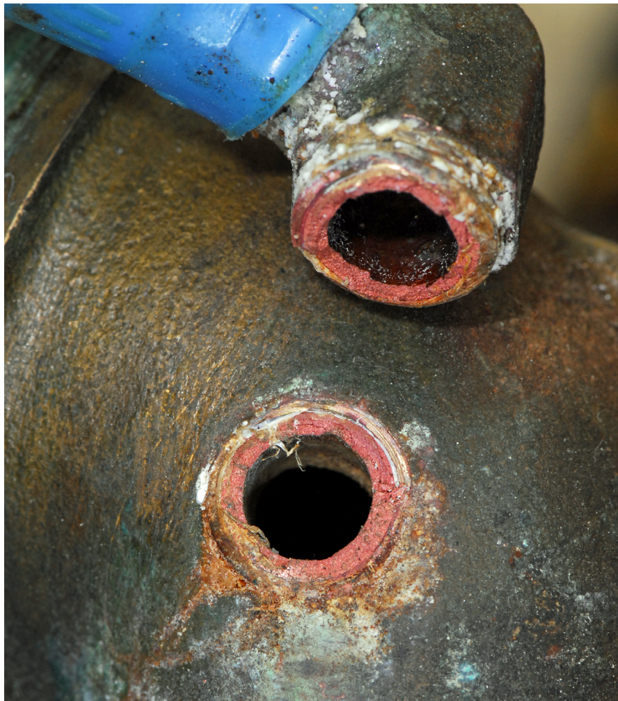
Brass is often inadvertently installed in pipe-to-hose adapters and pipe plugs in raw-water systems where it is vulnerable to dezincification.
