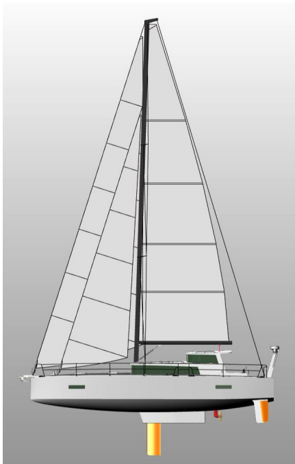
The EXP44 rig is a compromise between high performance and manageability for a small crew in challenging sailing conditions.
