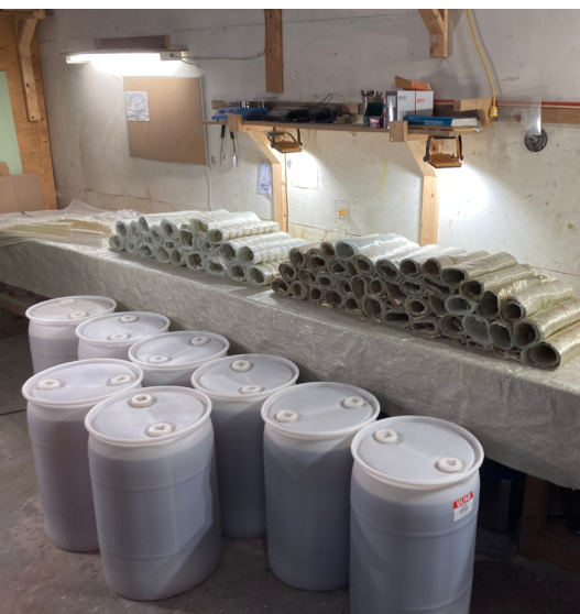
Rolls of glass reclaimed from a 20' (6.1m) section of wind turbine blade spar cap and the barrels containing the acetic acid solvent that dissolved the Recyclamine resin from the laminate.
