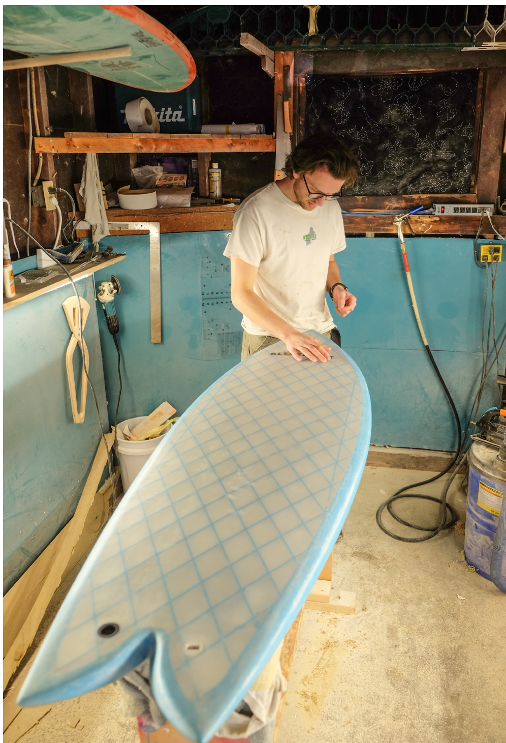
Builder Mike Ballin inspecting a Screaming Gull model board from Blueprint's line. Note the core vent and tether attachment points at the aft end of the board.
