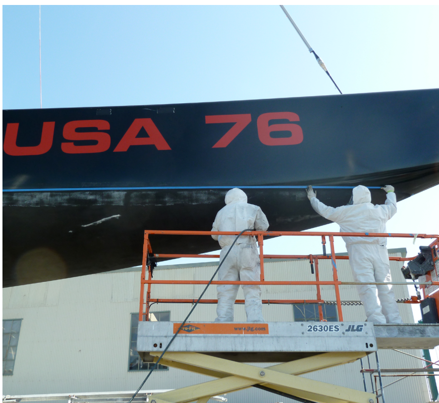
Taping the waterline assures a sharp line of transition between bottom and topside paints.
