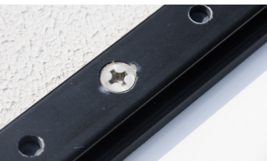
Aluminum sail and turning-block track on masts and deck are frequently attached with stainless fasteners, leading to mild galvanic corrosion.
