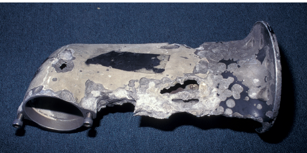
Aluminum lower units, common on stern, pod, and sail drives, are particularly vulnerable stray-current corrosion.
