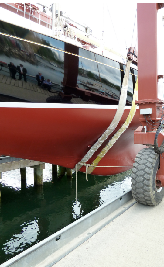
A coat or two of copper-based bottom paint is a standard annual maintenance measure, especially on traditional wood hulls.
