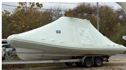
A standard service yard shrink-wrap application for boat storage includes a zippered door and air vents.
