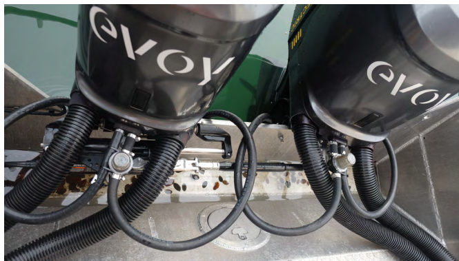
Under their cowling, each Evoy 120+ outboard houses an electric powerhead as well as water pumps, filters, and heat exchangers to cool the motor and batteries.
