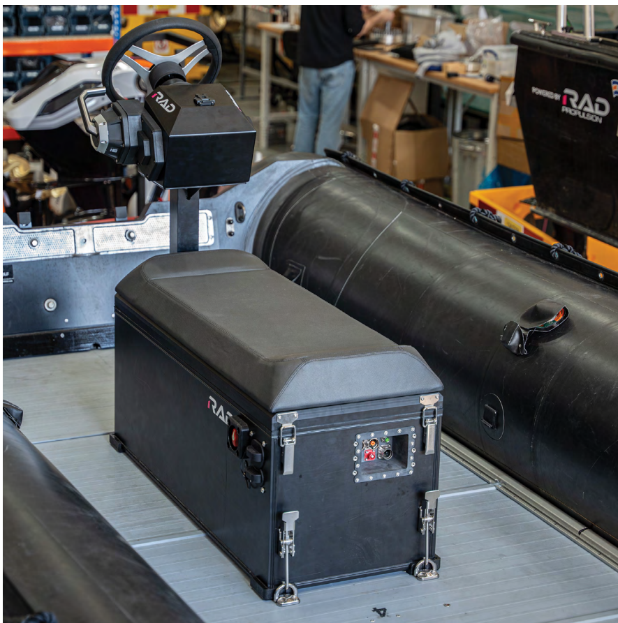
The combined drop-in battery box and steering console simplifies construction and systems installation for builders looking for an accessible electric propulsion option for smaller boats.
