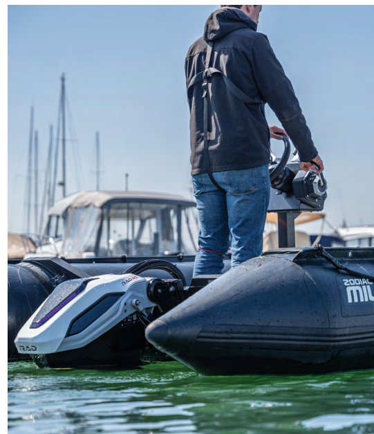
Left —RAD co-founders Dan Hook and Rich Daltry. Below —The RAD electric motor has a distinctive low profile which depends on its ability to be submerged in service. Installation is simplified by the fact that the fixed powerhead doesn’t need room to rotate in steering the boat.
