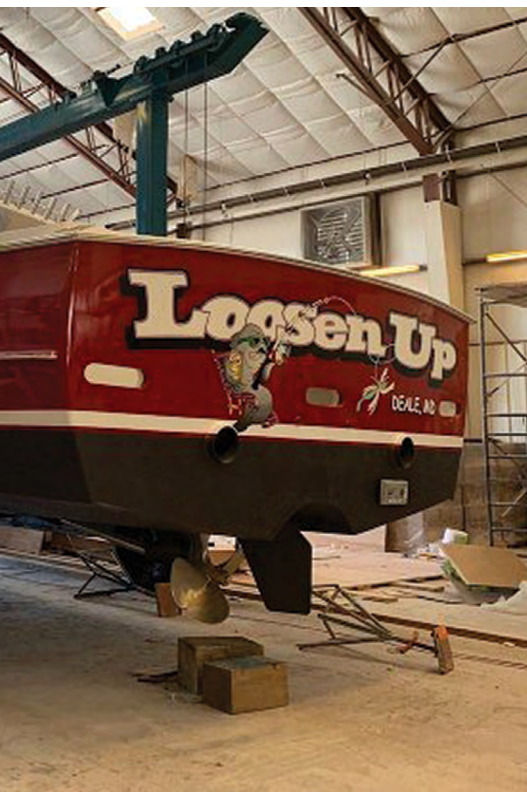
The centerline propeller tunnel reduces shaft angle and reduces draft while accommodating a large-diameter prop.
