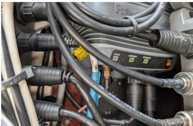
Left —The SXM receiver is buried somewhere beneath a host of other electronic components; note that none of the cables is labeled. Right —To access the SXM receiver, the VHF, AIS, and antenna splitter all must be disconnected and removed.
