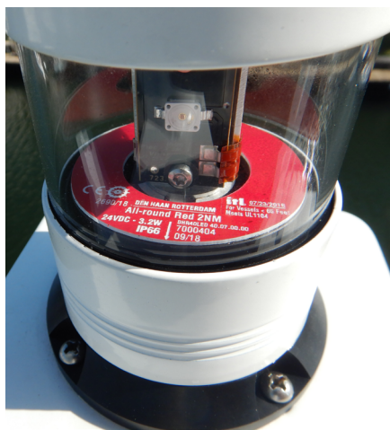
Be sure a light's rated range (2 nautical miles in this case) satisfies the Coast Guard's requirements for the vessel length.
