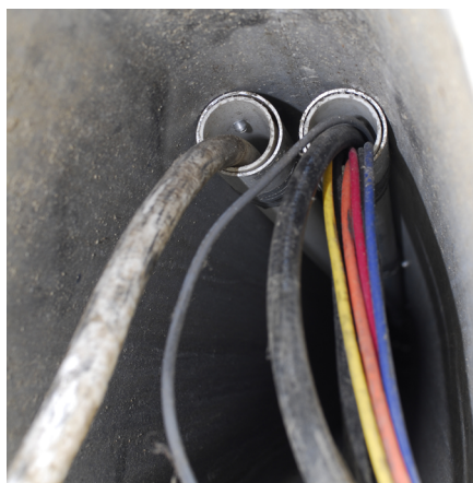
Left —Wiring inside of sailboat masts should be run through a conduit. Right —This wiring exiting the base of the mast is appropriately bundled and wire-tied but should have chafe protection where it bears against hard metal mast and frame structures.
