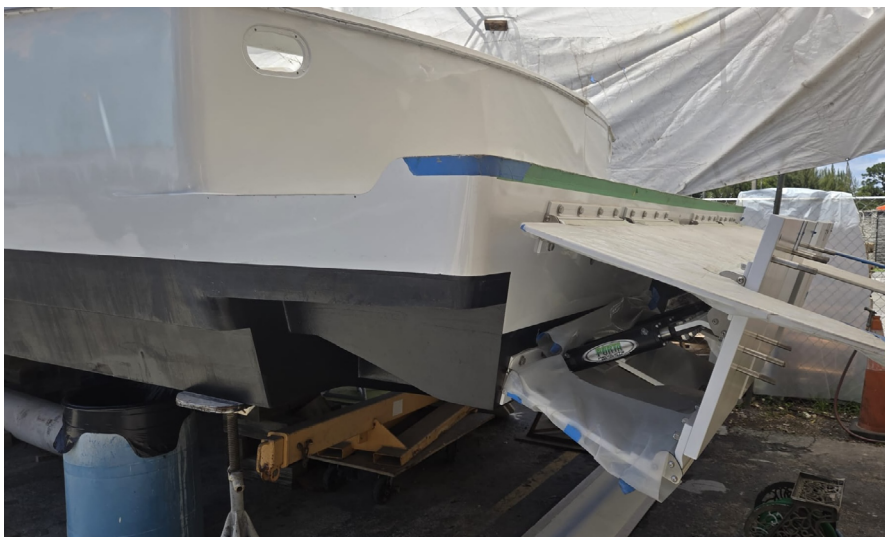
Left —For José Abella, converting the Viking is a hands-on exercise in experience- and intuition-driven design. Right —Accommodating four Mercury 600 outboards on a custom Porta bracket, the new transom also adds buoyancy and better lift when backing down.
