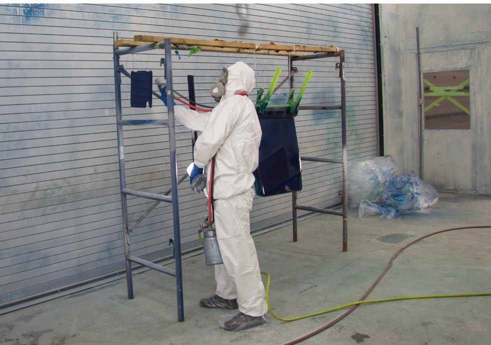
Left —At Front Street Shipyard, an applicator sprays individual boat parts, which offers an opportunity to test paint color and behavior before shooting a complete hull or house structure. Above —When boxing paint, applicators combine and mix all cans for a spray job ahead of time to even out any variations.
