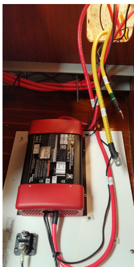
Left —Only one hand at a time can reach the essential electrical system components and connections in this compartment. Center —To improve access, the author installed the new equipment with extra wire length on a mounting panel. Right —Now, the new gear can be housed in the same space but be easily serviced by removing the panel.
