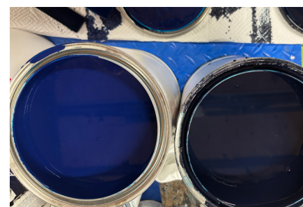
Top —Several gallons of midnight blue paint are opened and ready to be boxed. Bottom —A close-up of these two cans reveals clear color differences.
