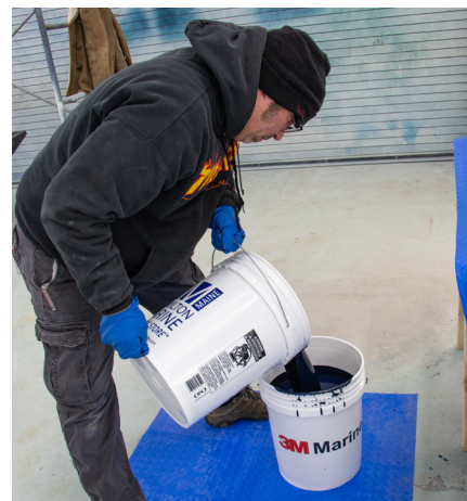
Left —At Front Street Shipyard, an applicator sprays individual boat parts, which offers an opportunity to test paint color and behavior before shooting a complete hull or house structure. Above —When boxing paint, applicators combine and mix all cans for a spray job ahead of time to even out any variations.
