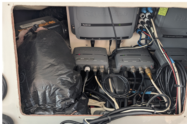
Left —The SXM receiver is buried somewhere beneath a host of other electronic components; note that none of the cables is labeled. Right —To access the SXM receiver, the VHF, AIS, and antenna splitter all must be disconnected and removed.
