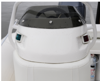
Left —Sidelights should be installed above the sheerline and be shimmed to ensure proper placement relative to the centerline. Right —Sidelights mounted on curved center consoles are often out of alignment and easily obstructed by passengers.
