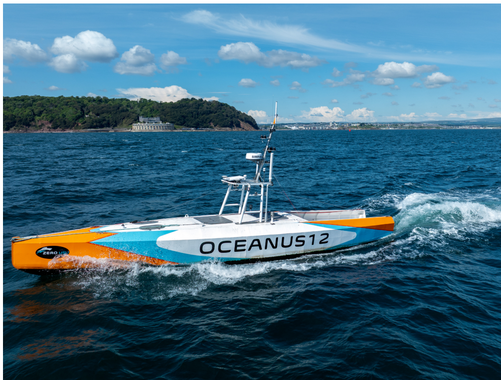
The Oceanus 12's narrow, long lines borrow from sailboat design to create an easily driven hull for maximum fuel efficiency and long distance capability.
