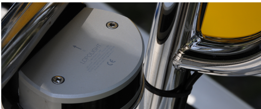
The fine print on this stern light specifies its compliance with COLREGS requirements; however, the adjacent stern rail support obscures the full arc of illumination, making the light noncompliant.
