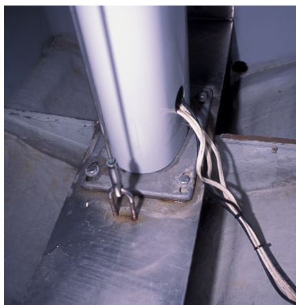
Left —Wiring inside of sailboat masts should be run through a conduit. Right —This wiring exiting the base of the mast is appropriately bundled and wire-tied but should have chafe protection where it bears against hard metal mast and frame structures.
