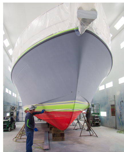
Days of prep work, including precise taping of bootstripes and meticulous hull sanding and priming, is critical to a paint job's positive outcome.
