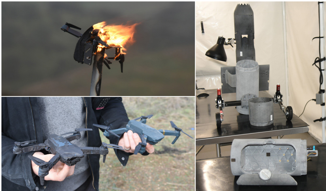
Top left: A Group 1 quadcopter burns after being engaged by Aurelius Systems’ laser weapon system. Bottom left: Side-by-side comparison of quadcopters with and without laser damage. Right: Modular airframe components of Firestorm Labs’ Tempest drone built by its xCell expeditionary additive manufacturing station. Naval Postgraduate School runs the quarterly Joint Interagency Field Experimentation event at Camp Roberts. Photo credit: U.S. Navy | Dan Linehan.
