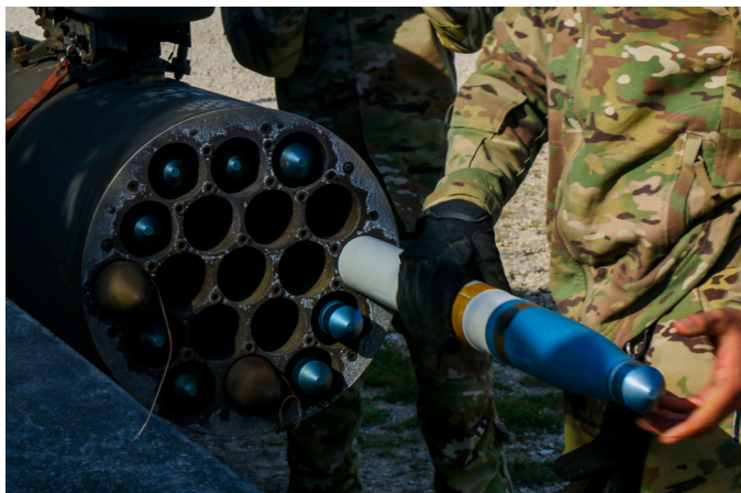
A U.S. Army Soldier assigned to the 12th Combat Aviation Brigade loads an Advanced Precision Kill Weapon System training round for a live-fire exercise, Sept. 23, 2021. The reloadable pod can house 19 rockets. Photo credit: U.S. Army | Pfc. Jesus Menchaca.
