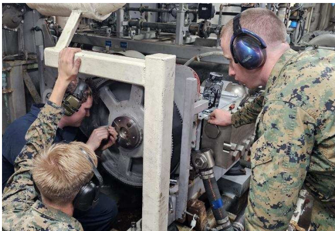
A U.S. Navy Sailor and U.S. Marine install a 3D-printed stainless steel component aboard the USS Somerset (LPD 25), July 18, 2024, during Exercise Trident Warrior 24 and RIMPAC 2024. Photo credit: U.S. Marine Corps.
