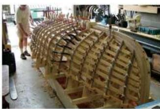
WELL BUILT STRONGBACK/ Mold for building the John Gardner Wooden 14' Sailing Whitehall. Includes a completed backbone. Has every plank spiling and patterns for every part. Includes loftings, jigs, clamp blocks, wedges, etc. Tooling was professionally made. These beautiful sailing Whitehalls won Best Professionally Built Whitehall at the 2010 WoodenBoat Show. Photos available. Asking \$1,000. 401–824–6585.
