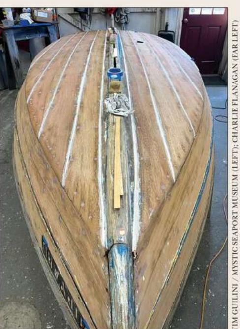
caulked," then prime-painted. As of this writing in late February, the boat had been turned upright and the coamings and foredeck were removed so that cracked deckbeams and the mast partner could be replaced with new ones of white pine, as specified in the designer's notes.
