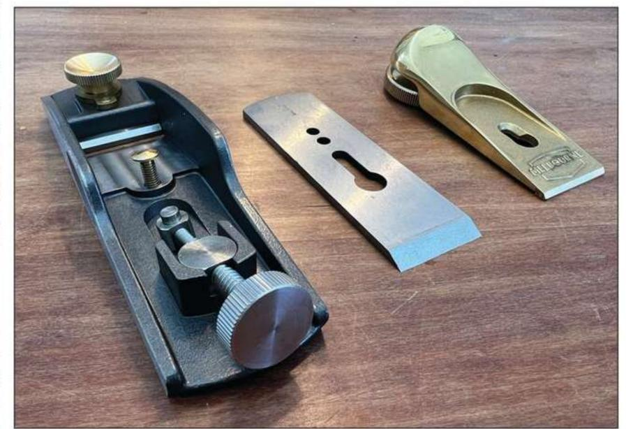
The cutting iron is made of high-speed steel and ground to 25 degrees. The brass lever cap that holds it in place is locked down by a knurled wheel.
