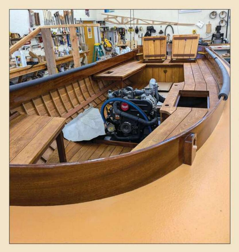
**15.** Attention then shifted to designing and building the interior. The Yanmar required a portside discharge instead of the starboard-side one shown in the plans—so the interior layout had to be essentially flipped, with seating planned to allow access and safe movement around the boat. The seats were framed in sapele, with cedar tops.
