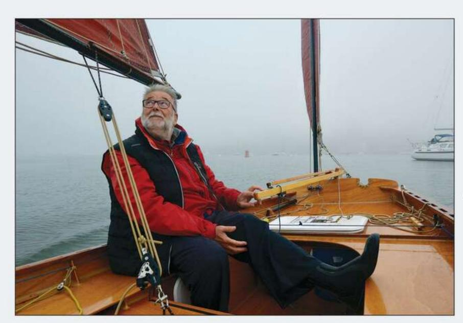
Emmanuel at the helm of the Grand Silmaril VITA BREVIS. For steering while sailing singlehanded, the helm has control lines on each side that run forward to the mast.
