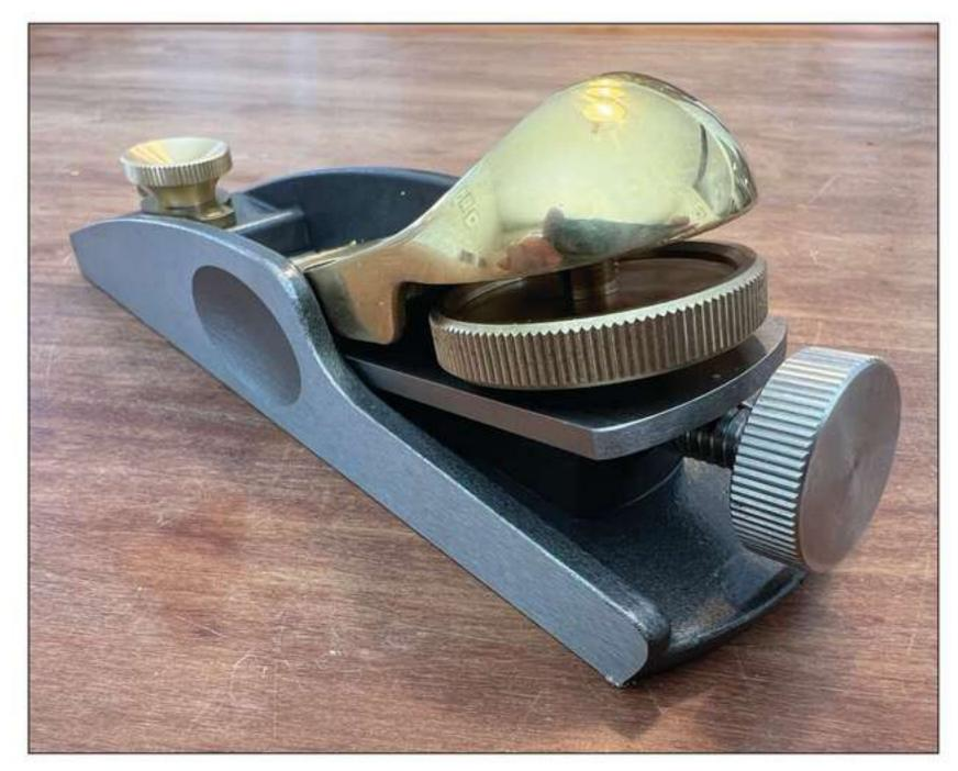
The depth-of-cut mechanism is precise, with little or no slop.
