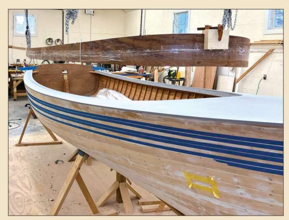
14. After the glue had set on the scarfs, the full-length coaming was lowered into place and installed as a unit. The top edge's shape was fine-tuned by using masking tape and sighting it from various angles, and subtle changes were made with a hand plane until it was fair and pleasing to the eye. When the fit was finalized, the coaming was glued and screwed in place.
