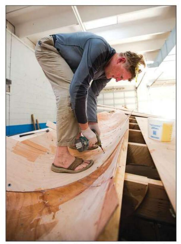
For TIMID TUNA, Bandy built a cold-molded tunnel into the hull bottom aft to accommodate the propeller-shaft's angle reduction from 12 degrees to 6 degrees.
