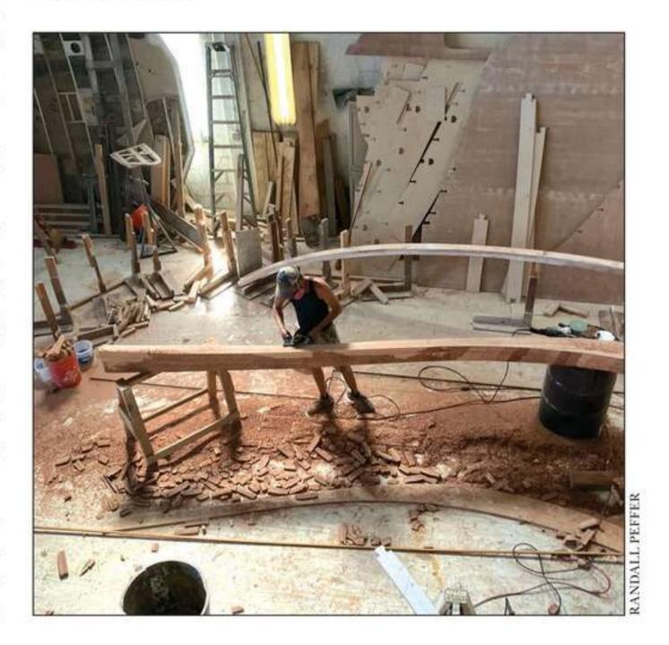
Even as PERLAMAR was launching, a 70-footer was nearly ready for hull setup, with bulkheads and molds standing by as keel assembly advanced.
