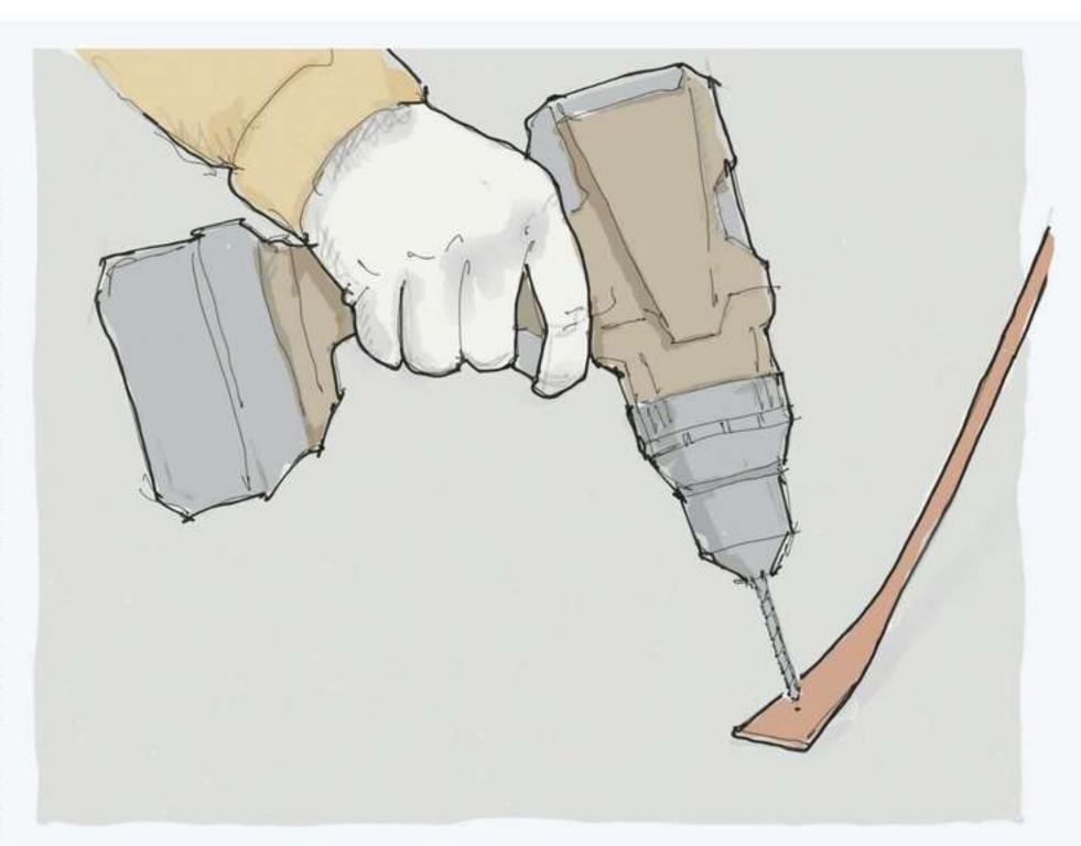
use a bit with at least a 135-degree split point, which tends to be selfcentering. This type of tip requires less force than a standard one when boring the metal.
