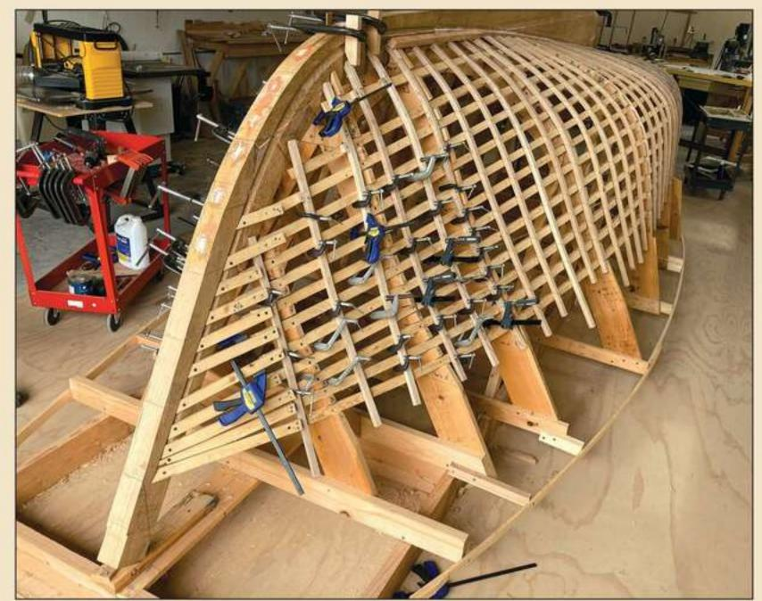
**5.** A local sawmill supplied green white-oak stock for the %"-thick × 1"-wide steam-bent frames. While fresh from the steambox, the frames were clamped over the ribbands and held in place with wire.
