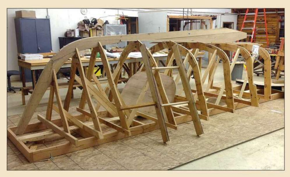
pieces were fastened together using bronze carriage bolts, with bedding compound applied to the mating, or faying, surfaces.
