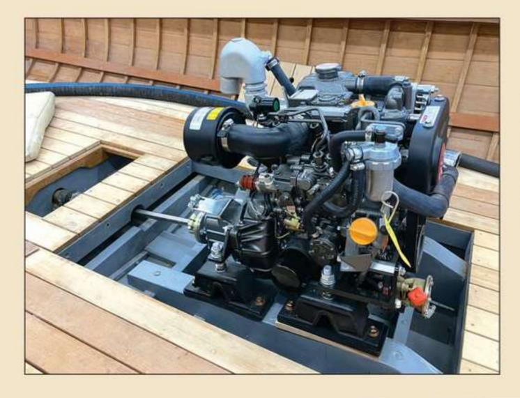
**12.** The Yanmar engine is very compact, but it was important to leave room for routine maintenance. The water pump is easily accessible, as are the dipstick and oil-fill tube. The radiator cap for the freshwater cooling is on the top of the engine. Sole hatches permit quick access to the stuffing box and the seawater valve and strainer.
